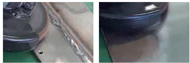
Removing blue weld discoloration Removing Rust
